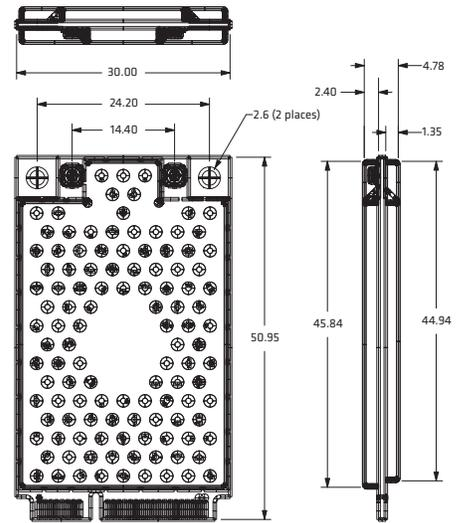
**IM11 RFID Reader Module Physical Specifications**
