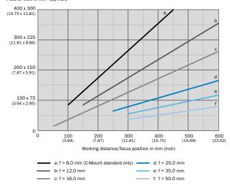
For S-mount and standard C-mount lenses, spacer rings are needed for working distances shorter than approximately 10 times the focal length. For compact C-mount lenses, spacer rings are not needed, but the built-in illumination cannot be used for distances shorter than 300 mm.
