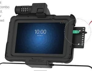
Optional accessory bracket allows you to connect RAM® 2-hole diamond bases for device mounting and features a cable management system for power cables or additional peripherals
