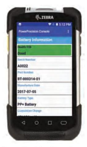
PowerPrecision Console provides all relevant information on the installed device battery required to identify and remove unhealthy batteries from the battery pool. Information is available on the mobile device and on the dashboard that can be accessed by virtually any device — desktop or laptop computer, tablet and more.
