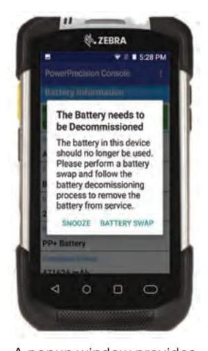
A popup window provides directions to users. You can allow users to 'snooze' the alert to swap the battery at a later time or require workers to complete the requested action in order to resume using the device.
