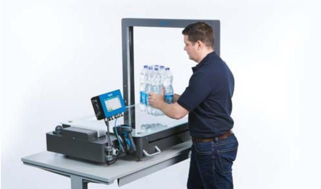
**1. Place the measuring object on the Master Data Analyzer measuring field.**
