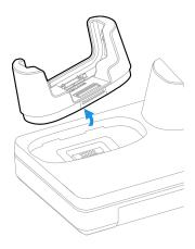
4. Insert the new cup tilted slightly towards the front of the base.
