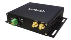
The RS200 is PC Based 2-port antenna RFID UHF fixed reader/writer for IoT applications. It is equipped with a wide range input power, USB, UART and 4 GPIO interfaces. With its compact design (100 x 89.4 x 27mm) this fixed reader/writer is not only applicable for RFID portals, but also suitable for POS self-checkout stations, kiosk services and product tracking and identity controls.
