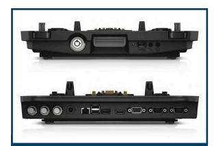
Front- and rear-facing port replication protects cable connections while integrated strain relief protects from accidental disconnects
