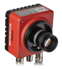
HAWK MV-4000 is a high-performance smart camera that boasts four times the processing power and six times the frame rate of the previous generation, making it a powerful option for all automation needs.
