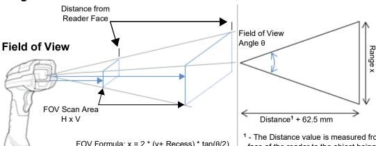
Note: The Recess value of 62.5 mm is the distance from the reader front face to the image sensor inside the reader. The Distance and Recess values are added together for the FOV Scan Area calculation.
