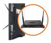
Choose the optional iiyama mini PC's with Intel® Core™ i5 inside to turn the displays into a stand-alone solution.
