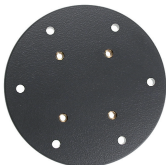
Item no. 215522 (black) 216522 (white) Mounting plate round Diameter 100 mm Thickness 9 mm AMPS-holes + 6 holes 4 screws + lock washers for attachment of base/top included.
