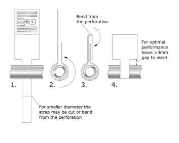
Ideal installation conditions are  $+20^{\circ}C$  ( $+68^{\circ}F$ ) / 50% RH. For exceptional conditions, please contact Confidex. Bond strength can be improved with firm application pressure.
