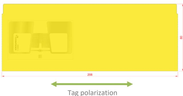
The label is delivered with no adhesive on the backside, so additional adhesive or plastic pockets are required for label attachment.
