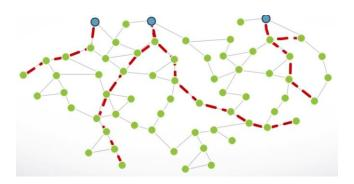
With Wirepas Massive, all devices can function as routers for other devices. Confidex Viking<sup>™</sup> Wirepas tags are suitable to be used both, as tags and anchors. Below described the main configuration parameters for Confidex Viking<sup>™</sup> Wirepas devices.
