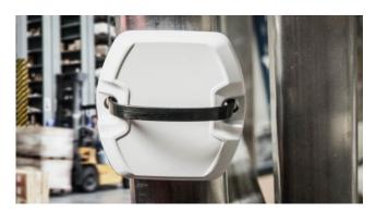
Plastic or metallic cable ties can also be used for fixing Confidex Viking<sup>™</sup>. Maximum width of cable tie is 4 mm.
