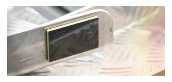
RFID tag with high temperature resistance and good performance for metallic surfaces
