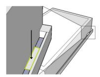
Ideal installation conditions are +20°C (+68°F) / 50% RH. For exceptional conditions, please contact Confidex. Adhesive of the label will provide best adhesion in 24 hours after the installation. Bond strength can be improved with firm application pressure. Always clean and dry the surface for obtaining the maximum bond strength.
