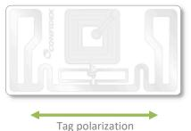
Ideal installation conditions are  $+20^{\circ}C$  ( $+68^{\circ}F$ ) / 50% RH. For exceptional conditions, please contact Confidex. Bond strength can be improved with firm application pressure. Always ensure clean surface for obtaining the maximum bond strength.
