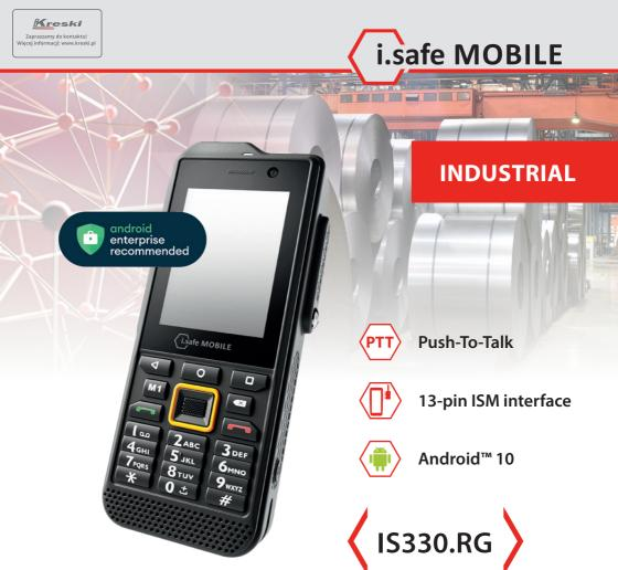
Thanks to the ISM interface, the professional PTT mobile phone for robust industrial use can be used like a radio device for connecting an RSM or PTT head-sets. The Android Enterprise Recommended device is zero-touch capable and can be managed via an MDM system. The particularly powerful loudspeaker and battery complete the highlights of this ultra-robust mobile device, which also has a good feel.
